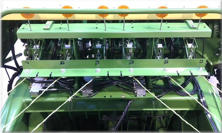
If a sensor (**S**) malfunctions while the machine is in operation, for example, you can deactivate knotter monitoring to stop the error message being continuously displayed.
