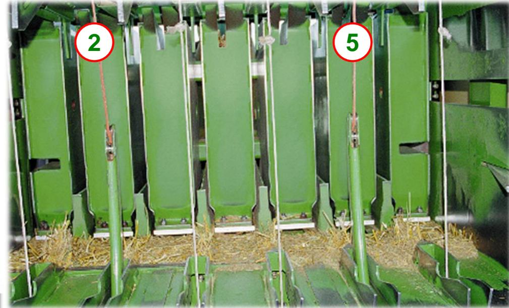
Six knotter needles are guided to the knotter via the automatically controlled ratchet mechanism to tie the big bale and the last MultiBale bale. Knotter needles 1, 3, 4, and 6 tie the big bale. Knotter needles 2 and 5 tie the last MultiBale bale of the big bale.
