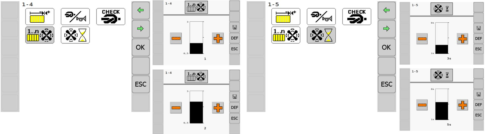
Knotter cleaning is performed shortly before the tying cycle. Depending on the operation conditions, the cleaning intervals can be set using the terminal in the menu "Settings/Knotter settings/Bale blowing" 1-4 between **0.5 all the way to every 3 bales**.
